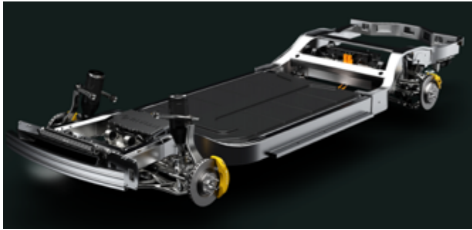
The 'skateboard' platform from the RIVIAN EV range afford compact storage and low center of gravity.
